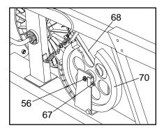
If the Belt (68) is properly adjusted, reattach the side shields and pedals. If the Belt needs to be adjusted, loosen the M8 Nylon Locknut (56) on each side of the Flywheel (70). To tighten the Belt, turn the two Adjustment Nuts (67) clockwise; to loosen the Belt, turn the Nuts counterclockwise. Make sure that the Flywheel is straight and tighten the M8 Nylon Locknuts (56). Reattach the side shields and pedals.
